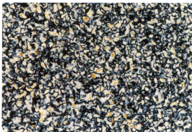
Figure 4. Microphotograph of the rectangular columnar (D ro ) mesophase of compound 2c between crossed polarizers; 1st cooling (1 K min -1 ) at 66°C.
